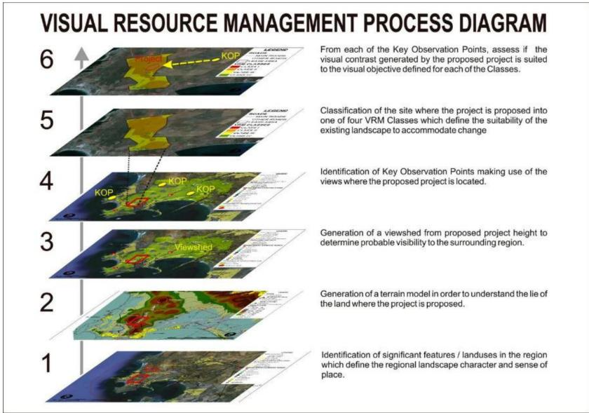
Figure 2: VRM process diagram
